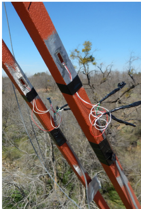
Figure 4: Strain gages on both eyebars of truss diagonal member.
