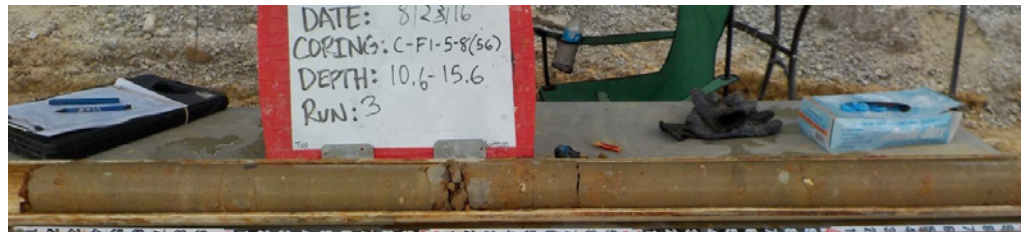
Figure 5: Typical Soil-Cement Mix Core Sample
