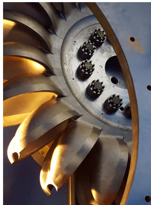
The pelton wheel inside its casing at the powerhouse.
