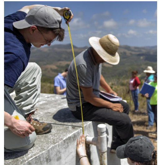
Mitchell Martin (EnvE, '22) measures the dimensions of an existing storage tank in our new partner community of La Pedregosa in Panama.
